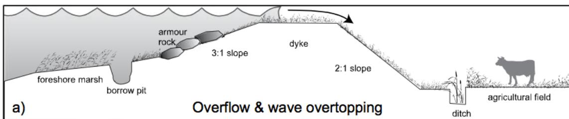
**Figure C2:** A type of mechanisms that can result in dyke failure, image taken from *Best Management Practices for Climate Change Adaptation in Dykelands: Recommendations for Fundy ACAS Sites*
