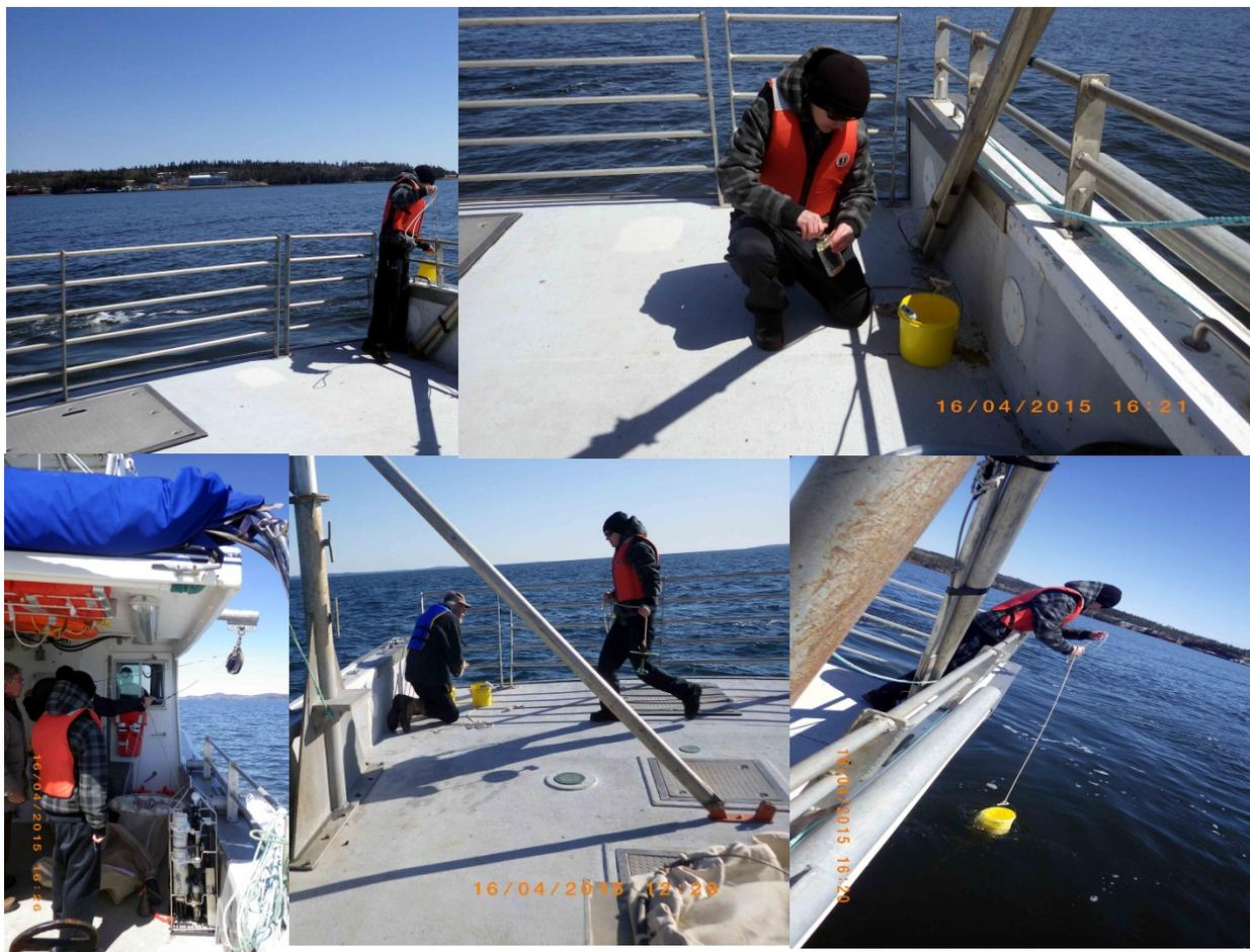
Figure 2. Hydrographic monitoring at station Prince 6. Clockwise from the upper left; Biological Station in background, surface salinity sample, collecting surface water, carrying Secchi disc across deck and CTD profiler deployment preparation.
