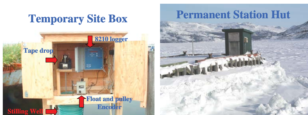
Figure 2. Temporary and permanent gauge stations
