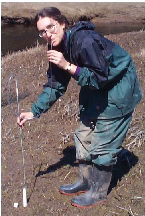
Figure 2. Using a metal and plastic tubing apparatus to determine depth to groundwater along a piezometer transect.
