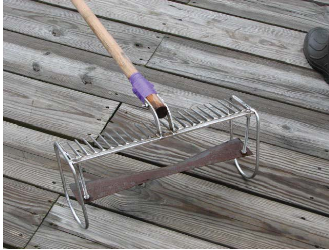
Figure 2. Cutter rake used for commercial harvesting of rockweed, Ascophyllum nodosum
