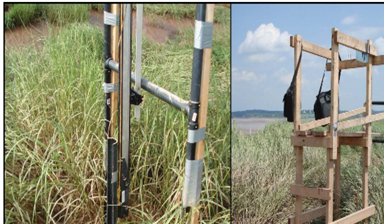
Figure 1. Photographs of the vertical sliding mechanism (left) and the personnel stand on the marsh surface
