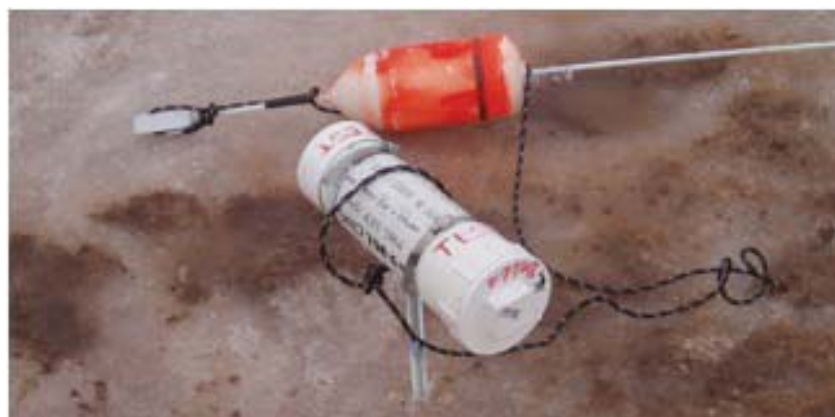
Figure 2. GPS ice tracking assembly (as installed)
