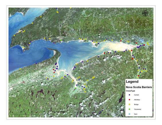
*Figure 12:* Example of map produced using a simple 'crossing type' query for tidal barriers in the Southern Bight overlaid on Landsat 7 base image. Data could just as easily be displayed over planimetric base map layer.
