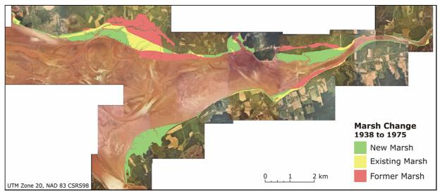
*Figure 14: Example in Cobequid Bay, NS of type of historical spatial analysis (quantification of change in marsh area) that can be conduced using this GIS database. Figure from Baker and van Proosdij, 2004.*
