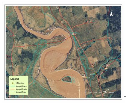
Figure 10: Magnified 4 m resolution digital orthophoto illustrating planimetric reference layer and tidal barriers.
