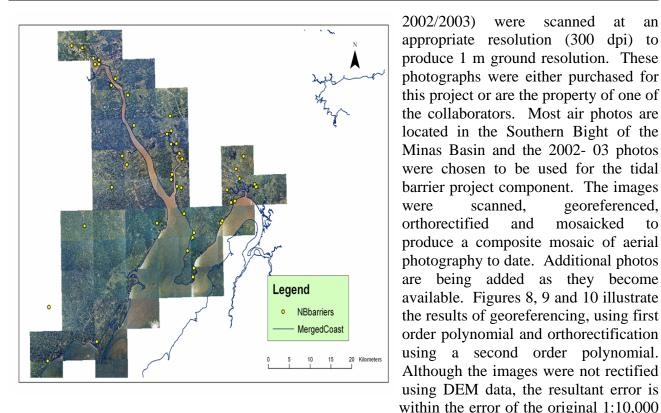
Figure 9: Initial (prior to refinement) mosaic created using NB digital orthophotographs available on-line at 4 m resolution.
