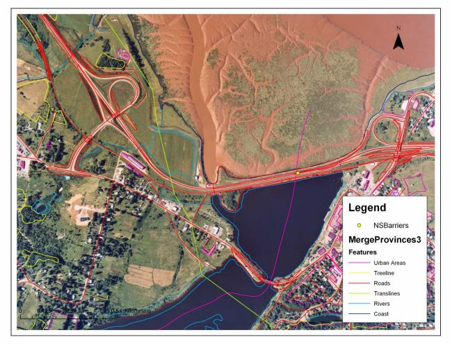
Figure 8: Planimetric vector data used to rectify air photos by collecting Ground Control Points and accurately aligning specified features
