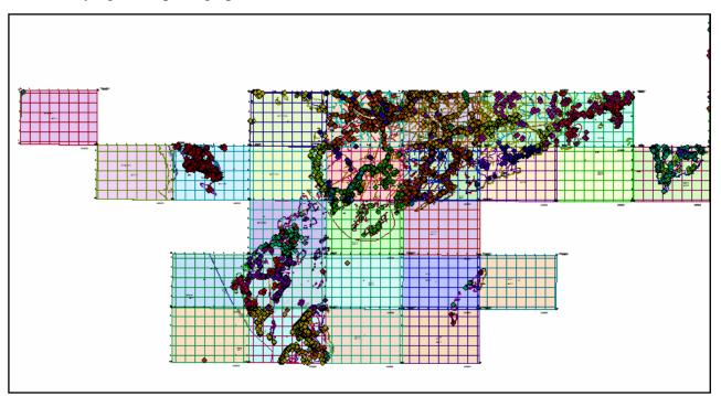
*Figure 4:* Example of 1:10,000 digital map sheets for southern portion of NB from Service New Brunswick. Data in the raw form is very cluttered and must be 'cleaned' prior to use.
