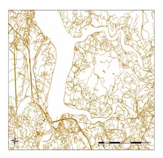
*Figure 5: a)* Avon river planimetric file without individual features is difficult to identify. This makes georeferencing and orthorectification very difficult.
